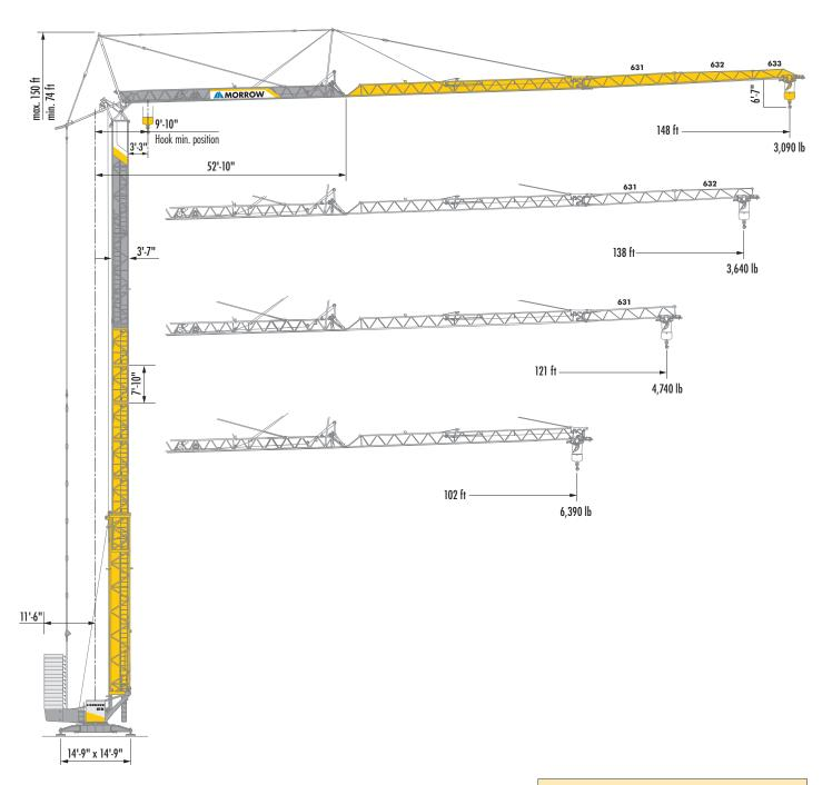
**IMPORTANT:** Consult 81 K Instruction Manual before erecting, operating, servicing and dismantling crane.
