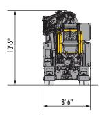
King pin towing assembly - double axle  $52,840\ lb$
