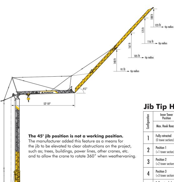
Some crane configurations do not allow 45° luffing. (See Stability section of the 81 K Instruction Manual).
